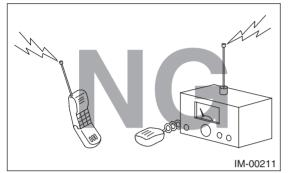
• When turning the ignition switch to ON or OFF while diagnostic items are being checked, do not allow keys with different ID codes close to the ignition switch. If the ignition key is on a key holder, remove it from the key holder before performing diagnoses.
