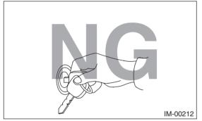
• When repeatedly turning the ignition switch to ON or OFF while diagnostic items are being checked, it should be switched in cycles of "ON" for at least 5 seconds  $\rightarrow$  "OFF" for at least 8 seconds.
